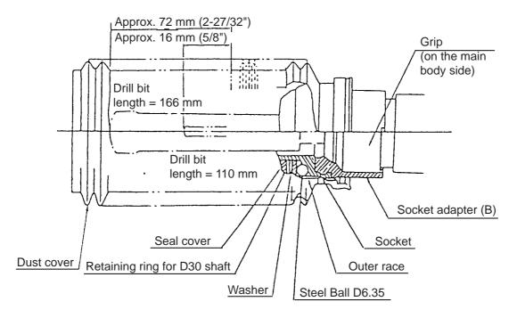
Fig. 7 Dust collector (B) structure
