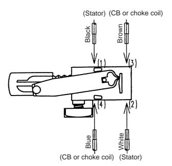
Fig. 18 Wiring of reversing switch
