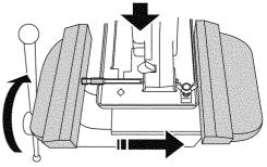
2. Loosen the depth adjusting nut and remove the spring washer and square screw from the depth adjustment nut.
