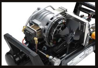
It has a dual-cylinder that takes air through 2 stages to make the air pressed up to 34bar by using the DC brushless motor. This compressed air provides power to the nailer and can drive through wood, concrete and steel. Inverter control allows it to operate in a low voltage situation from 140V up to 265V.
